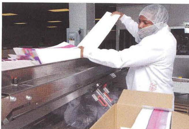
The high-capacity 72-in.-long powered carton magazine is ergonomically positioned at a comfortable height for loading.
