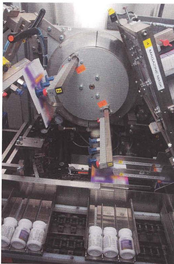
MGS’ vacuum carton pre-break and rotary carton setup mechanism ensure every carton is set up properly every time.
